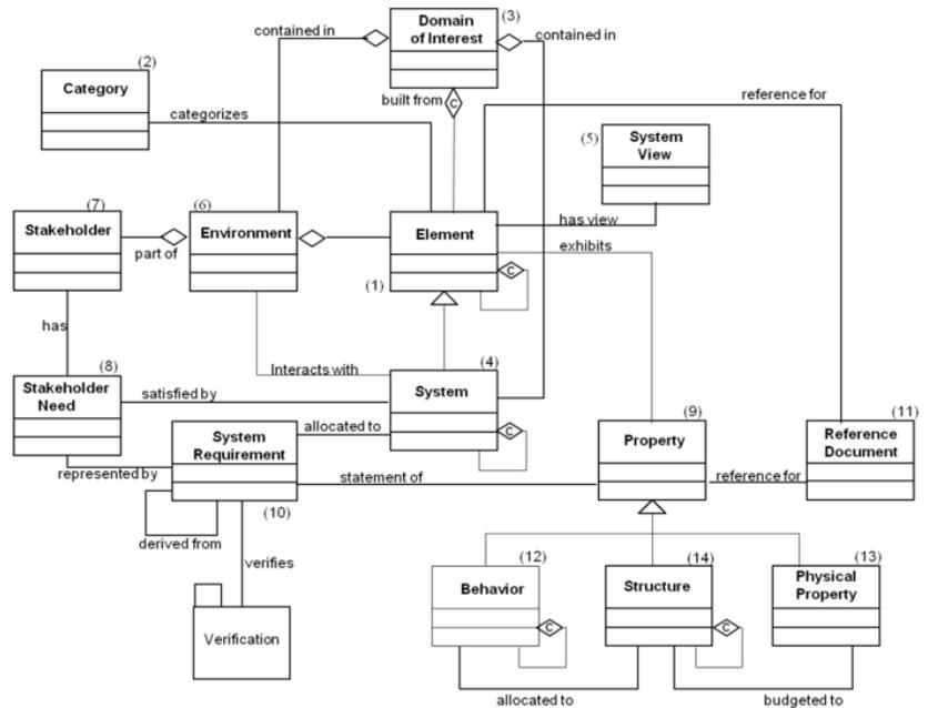
**Figure 1. Fragment of the Object Management Group System Concept Model (Oliver 2003, Slide 3).** Permission granted by David Oliver on behalf of INCOSE MDSD Working Group. All other rights are reserved by the copyright owner.
