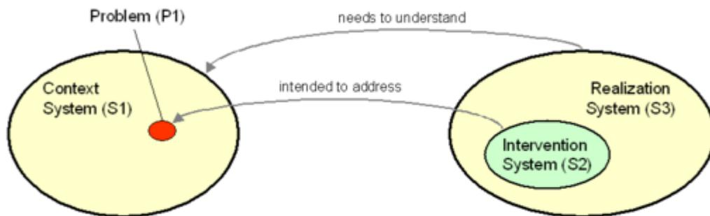
**Figure 3. Realization System That Creates the Intervention to Solve a Problem (Martin 2004).** Reprinted with Permission of Aerospace. All other rights are reserved by the copyright owner.
