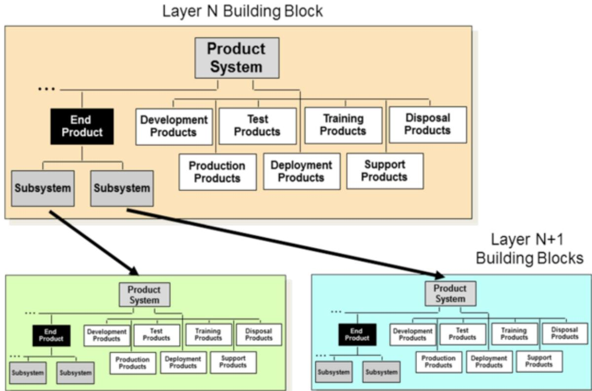
**Figure 2. End Products and Enabling Products (ANSI/EIA 632).** Excerpts from "Processes for Engineering a System" (EIA-632), Copyright © (1999) TechAmerica. All Rights Reserved. Reprinted by Permission. All other rights are reserved by the copyright owner.
