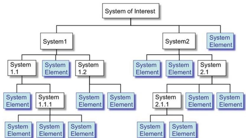
**Figure 4. Hierarchical Decomposition of a System-of-Interest (Faisandier 2012).** Permission Granted by Sinergy'Com. All other rights are reserved by the copyright owner.
