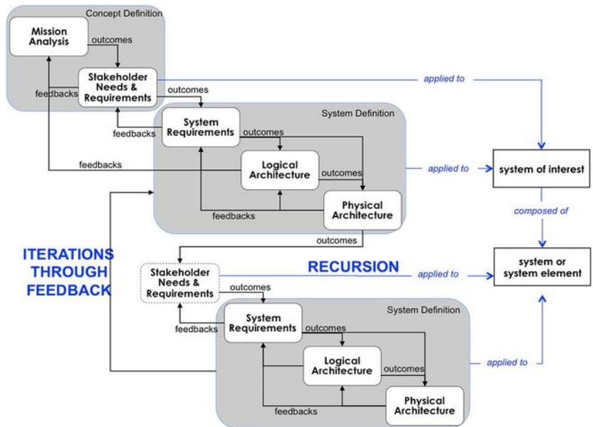
**Figure 5. Recursion of Processes on Layers (Faisandier 2012).** Permission Granted by Sinergy'Com. All other rights are reserved by the copyright owner.
